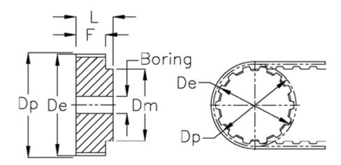
Belt width = - 25 mm = 75.15 De Dm = 50 = 76.4 Dp F = 30 L = 36 Pre-drilled = 8 Tooth number = 48
